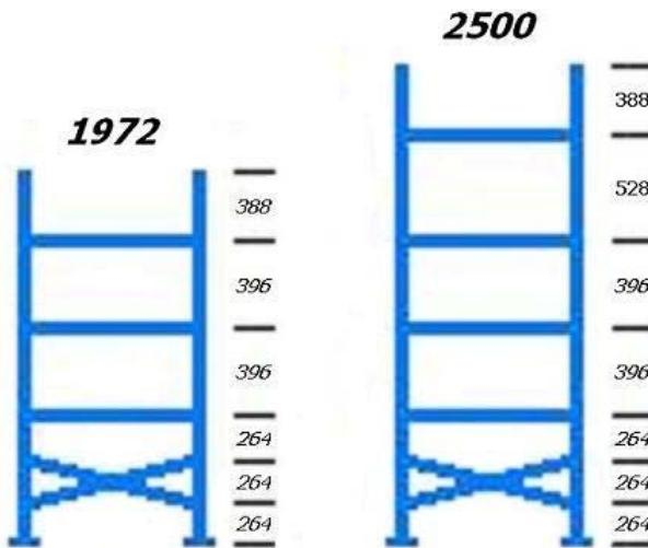
Insert the horizontal and diagonal spacer bars into the grooves in the corner of the upright, locating the wide part of the slot over the nibs on the upright. Keeping the spacer bars tight to the upright in order to keep it square, tap down into the narrow part of the slot, alternating from side to side. To achieve correct assembly, the spacer bar anti-release tongues should be closed\*.
