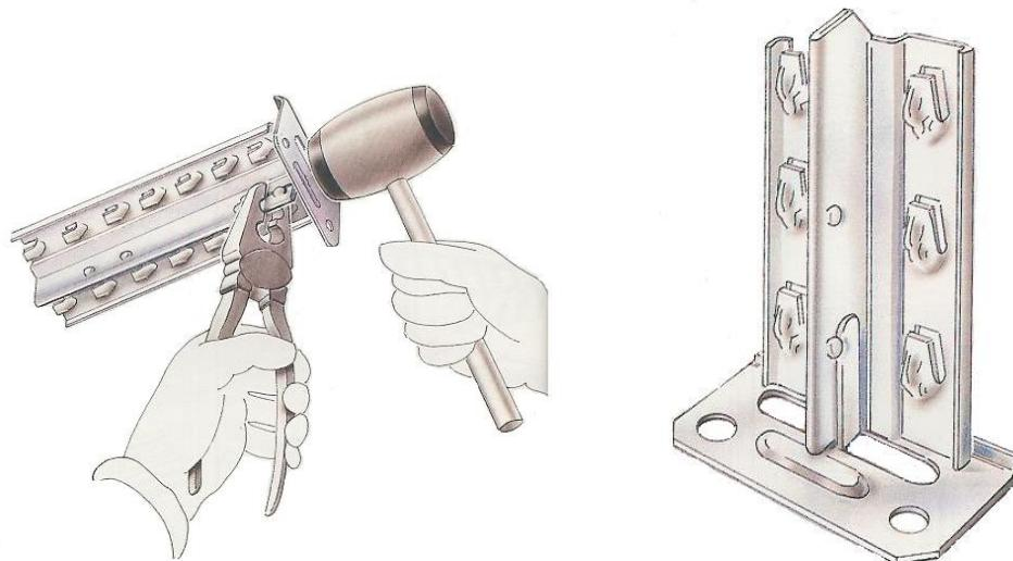
Alternatively, heavy duty base plates must be used in the following cases:
